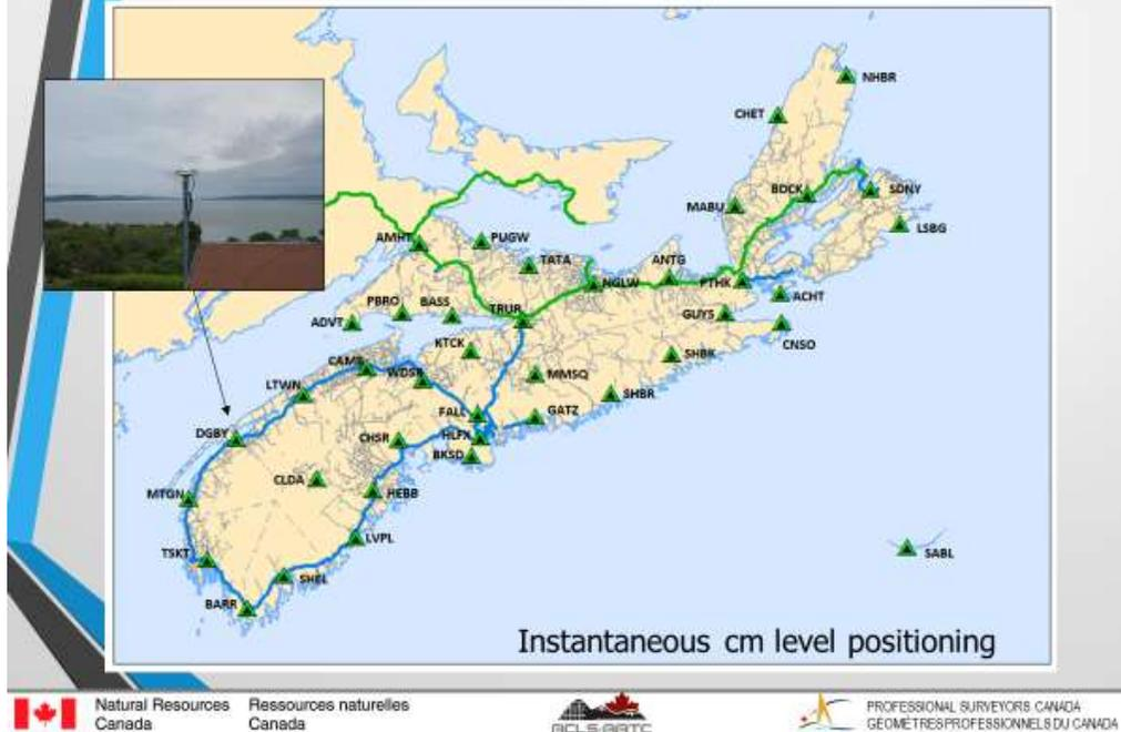
The Nova Scotia Active Control System consists of 40 active control stations, spaced at approximately 50 km to enable centimetre level positioning across the province in real-time. Areas without cell coverage can be served by accessing the archived data free of charge through CGS's website. Data from all of the stations is licensed to service providers so that they can offer high accuracy positioning services.
