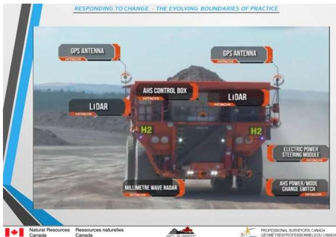
This technology has spread to construction sites as well, with autonomous equipment just entering the market. Again, a byproduct of this technology is the continual mapping of a site, providing real time as-built data, in addition to actually completing the task at hand.
